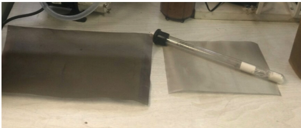
Fig. 3 SS US 100 wire with/without a thin film of ZnO photocatalyst.
